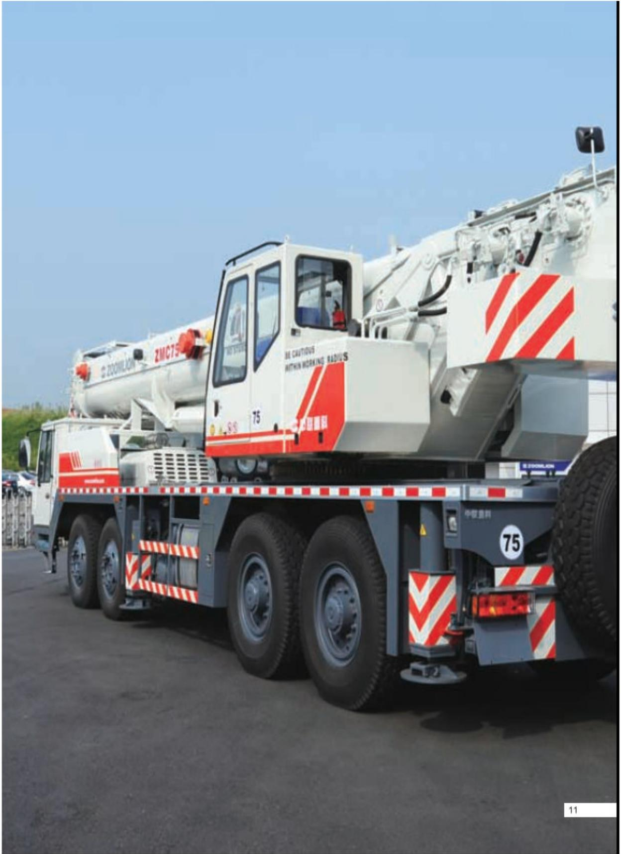
The lifting capacity fulfills the requirements of standard DIN 15019 part 2 with regard to stability.
